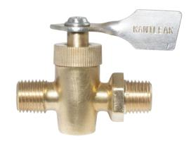
The 170 Series 2-Way Shut-Off Plug Valve features instantaneous onoff operation. This series has a solid bottom and is O-ring sealed. The O-ring seal, unlike packings, require no maintenance. The lapped brass body and plug are individually mated to provide an excellent seal. Generally recommended for gasoline, oil, kerosene, LP gas, gasair mixtures, and air system applications.
