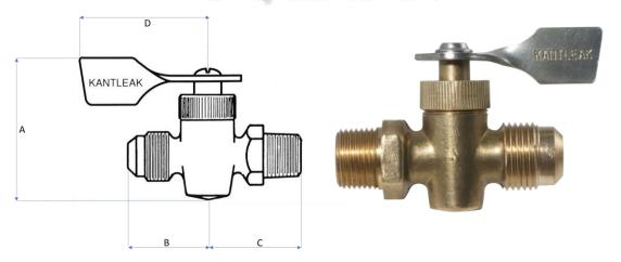
The 170 Series 2-Way Shut-Off Plug Valve features instantaneous onoff operation. This series has a solid bottom and is O-ring sealed. The O-ring seal, unlike packings, require no maintenance. The lapped brass body and plug are individually mated to provide an excellent seal. Generally recommended for gasoline, oil, kerosene, LP gas, gasair mixtures, and air system applications.
