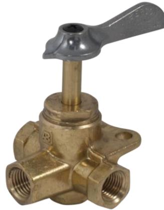
The 110 Series non-lubricated selector valves are designed to operate in systems where instantaneous port selection is desired. Since lubricants are not used, re-lubrication is not required. There is no lubricant to freeze and lock the valve or to contaminate fine fluids. The O-ring sealed cap and stem eliminate leakage. The series is designed for panel or bracket mounting. Standard with pointer lever to indicate the desired porting selection and can be rotated 360 degrees.
