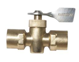
The 170 Series 2-Way Shut-Off Plug Valve features instantaneous onoff operation. This series has a solid bottom and is O-ring sealed. The O-ring seal, unlike packings, require no maintenance. The lapped brass body and plug are individually mated to provide an excellent seal. Generally recommended for gasoline, oil, kerosene, LP gas, gasair mixtures, and air system applications.
