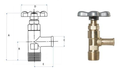
**97 Series** Rising Stem Valves are used extensively in the industrial, heavy duty construction equipment and mobile fleet markets. They are high flow valves recommended for operation with gasoline, oil, kerosene, LP gas, gas-air mixtures, cooling systems and air systems.
